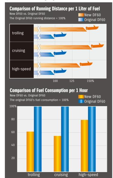
Data used in the graphs were obtained through in-house testing under uniformed conditions. Results will vary depending upon operating conditions (boat design, size, weight, weather, etc.)
